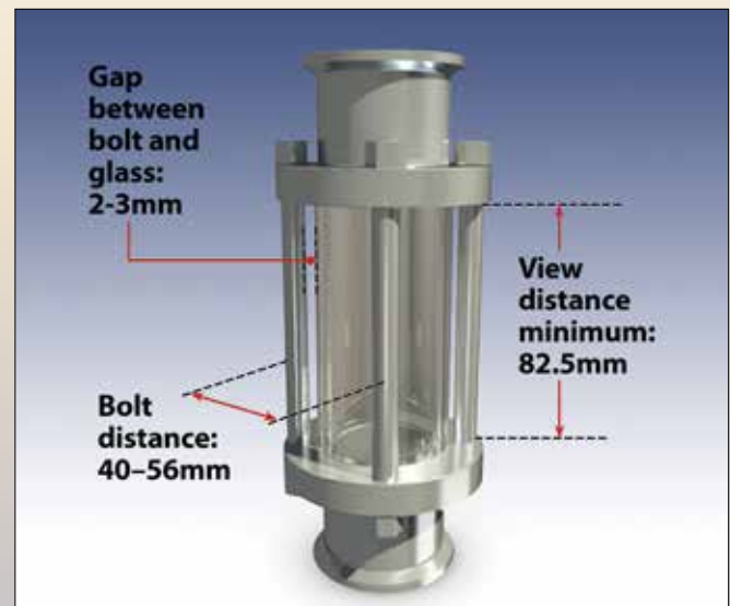
Sight Glass Dimensions for Optimal LumiFlo Light Fit
