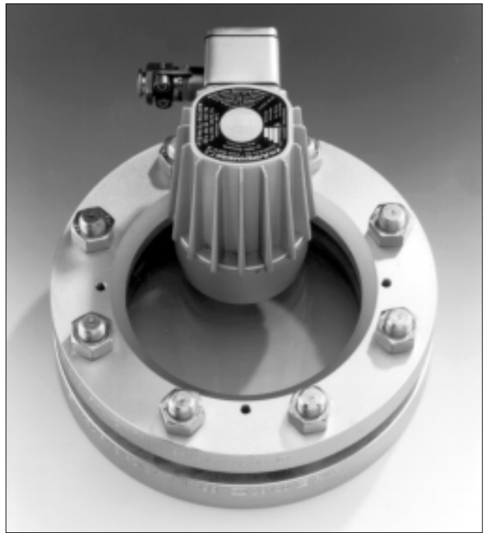
Lumiglas USL 06-Ex installed by a hinged bracket on the cover flange of a circular fitting DIN 28120, forming a combined sight/light port.
