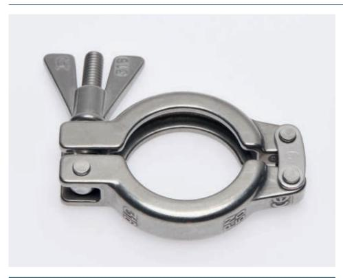
The **SH Safety Clamp** is based on the design of the widely accepted 316 stainless steel SH clamp, which includes the 'Omega' internal profile geometry known for its exceptional clamping efficiency. The SH style Safety Clamp's unique feature is the lower portion of the bolt is wider than the opening in the clamp's gate. In use, the wing nut must be deliberately loosened so the clamp gate can be lifted above the wider part of the bolt before the clamp can be completely opened.
